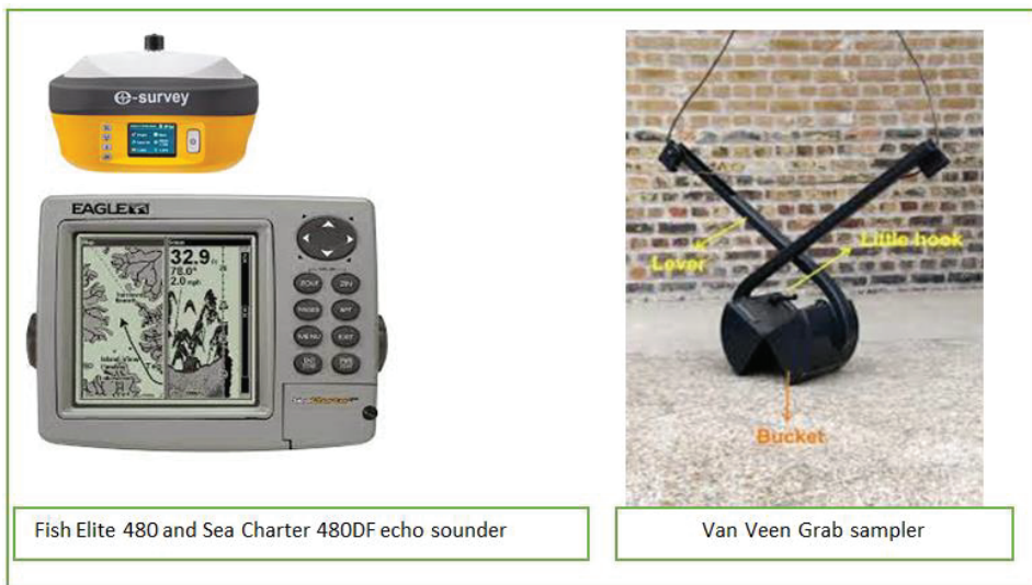
Fig. 1. Fish Elite 480 and Sea Charter 480DF echo sounder and Van Veen Grab sampler
