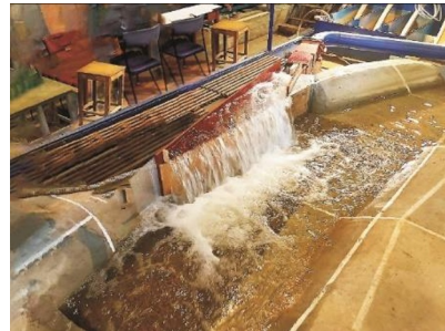
Fig. 5. Photos of laboratory studies of hydraulic modes of water well
