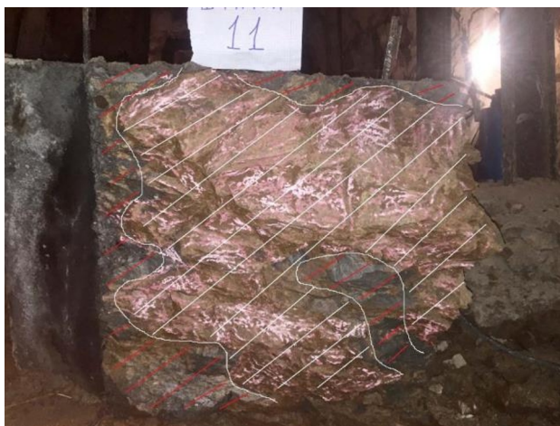
Fig 5. Shear surface after testing dies No. 11.
