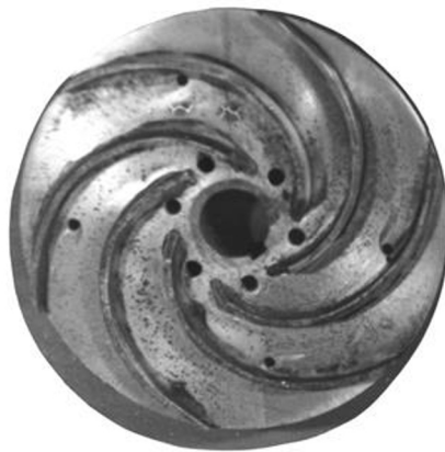
Fig. 1. Characteristics of 3K-6 with centrifugal pump n_0 = 2900 rpm (a) and its collapsible impeller (b)
