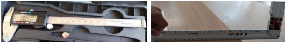
Fig. 2. Measuring and determining the difference between the plates using an electronic caliper and protractor.
