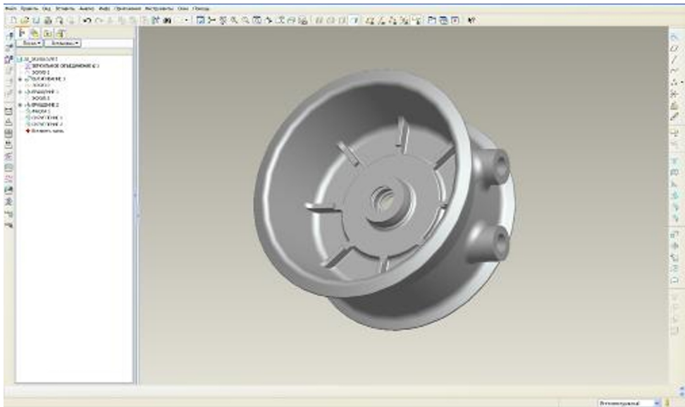
Fig. 1. Three-dimensional model of the brake chamber housing
