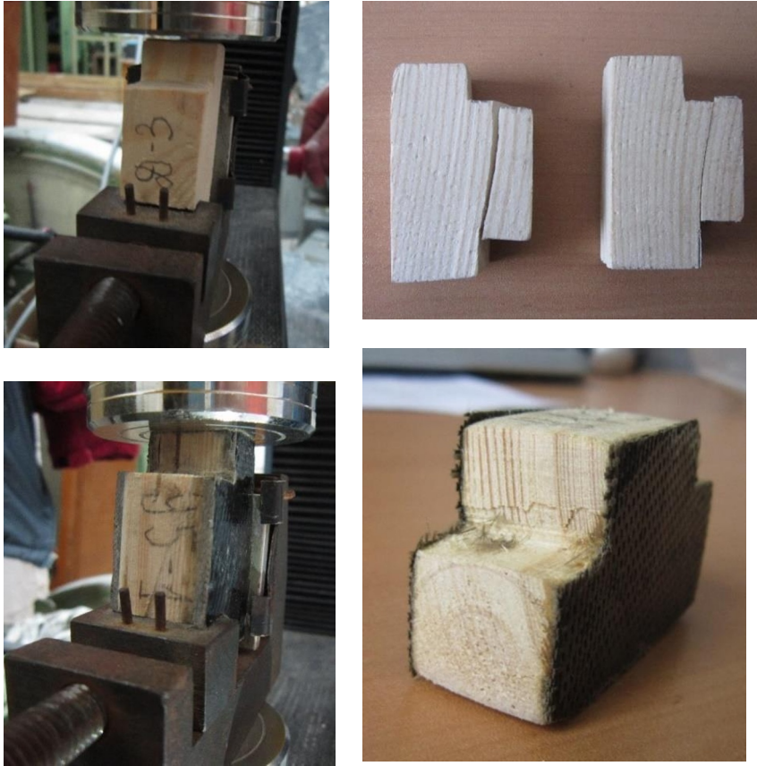
Fig. 2. General view of test and tested prototypes for shearing along the fibers.
