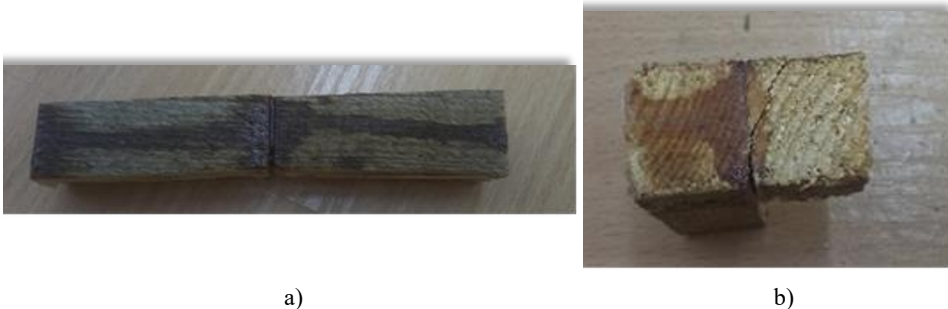
Fig. 5. Testing wood for adhesive strength of a polymer composition based on epoxy resin: a) in bending; b) in shear
