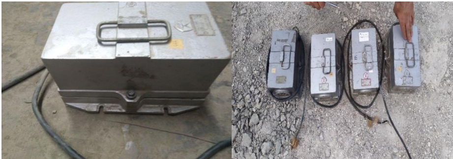
Fig. 1. Sensors for determining main oscillation parameters in three main coordinate systems x, y, z .
