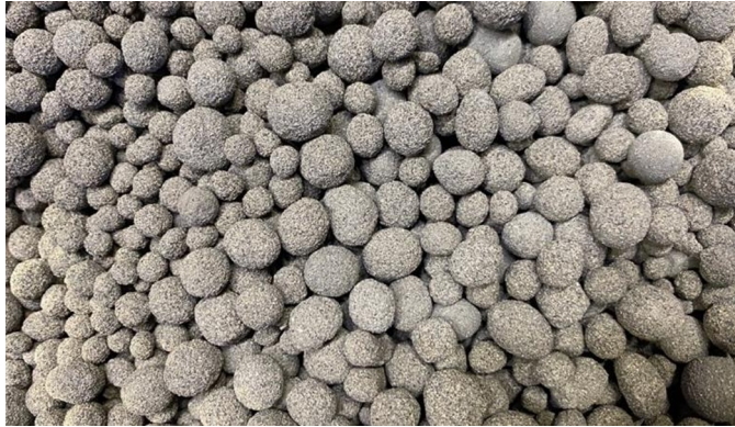
Fig. 1. Cold-bonded fly ash aggregate based on fly ash from Berezovskaya Thermal Power Plant.
