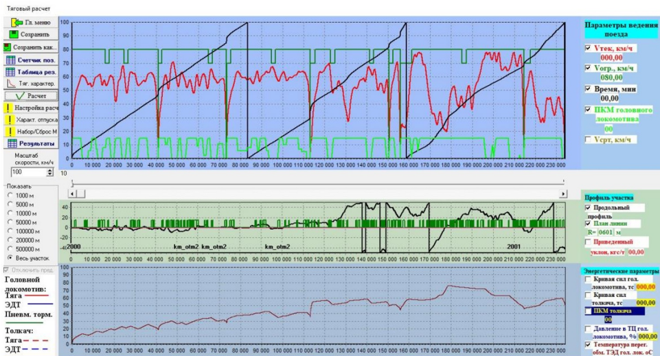
Fig. 2. Modeling a trip using the program "traction accounting"
