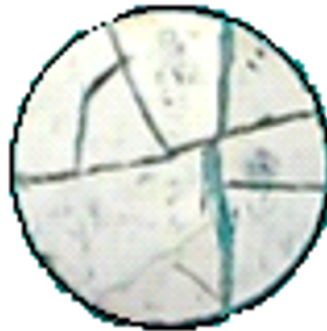
Fig. 3. Photocell surface image with damaged aluminum electrode
