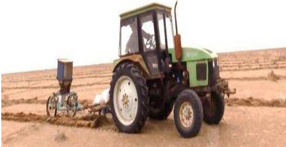
Fig. 2. Process of sowing seeds of saxaul and cherkez using experimental seeder (side view)
