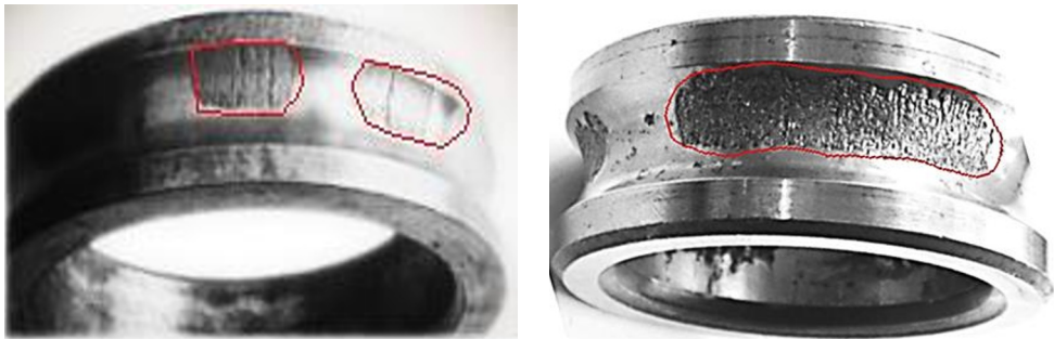
Fig. 3. Example of development of defect on outer ring of rolling bearing
