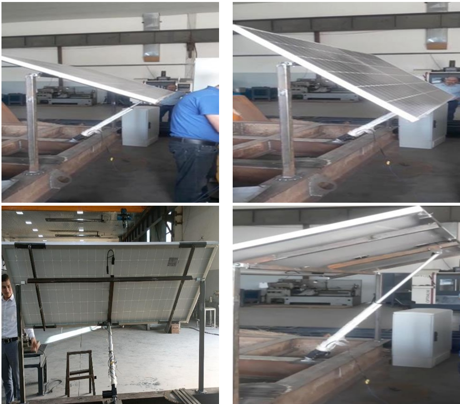
Fig. 2. General view of proposed solar tracker.
