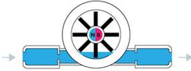
Fig. 7. YF-S201 Hall transducer operation
