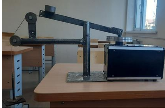
Fig. 2. Device that measures wear resistance
