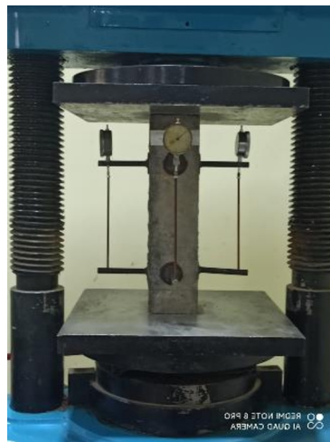
Fig.2. Overview of concrete prism testing
