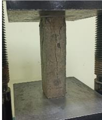
Fig. 9. General view of prism-sample with basalt fiber addition after test
