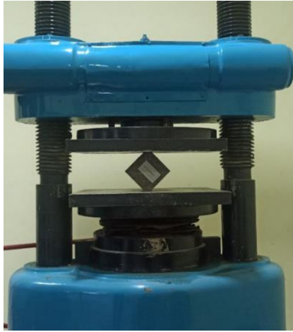
Fig. 7. Testing cubes for tensile strength in cracking
