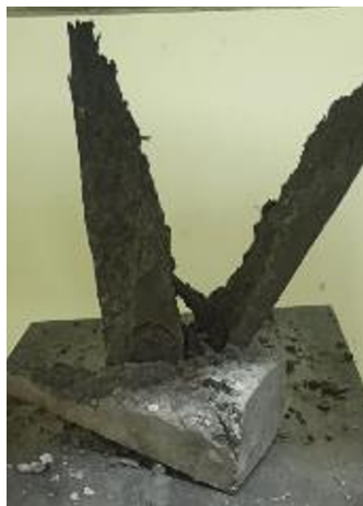
Fig. 8. General view of prism-sample without basalt fiber addition after test
