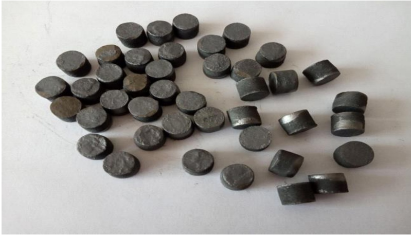
Fig. 9. Obtained high-pressure synthesis samples (without machining)
