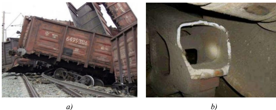
Fig. 1. Emergency on railway (a) as result of destruction of the cast side frame (b)
