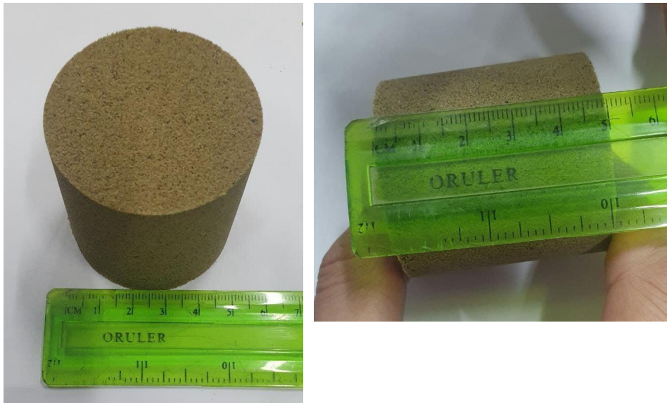
Fig. 3. Prepared specimens according to GOST 23409-78 with dimensions 50 x 50 for testing
