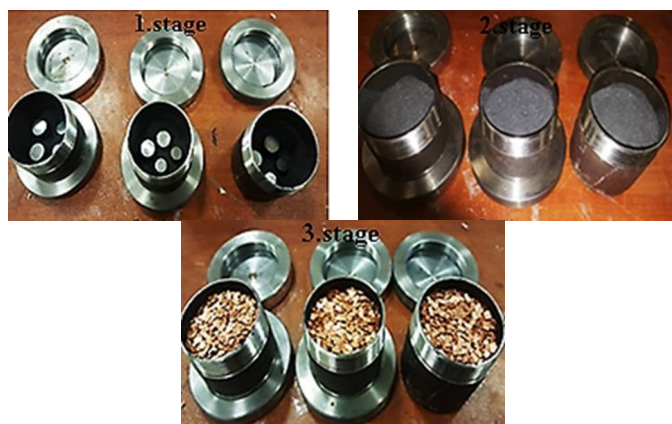
Fig. 1. Box boriding process stages
