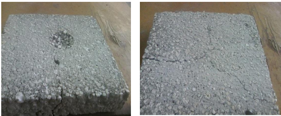
Fig. 3. The nature of the destruction of the control (H-4) sample
