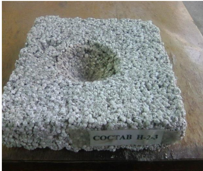
Fig. 5. The appearance of the sample H-2 after the impact strength test
