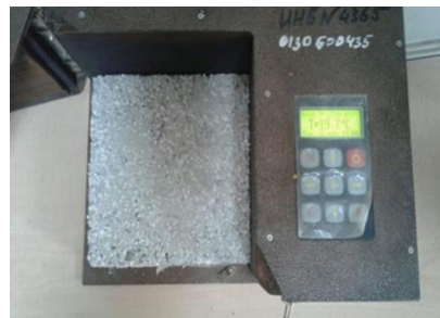
Fig. 2. Thermal conductivity testing of samples
