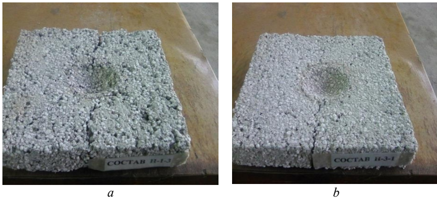
Fig. 4. The nature of the destruction of the sample H-1 (a) and H-3 (b)
