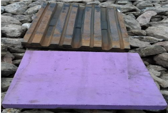
Fig. 1. Standard gasket TsP-204-M-ARS (standard, from above) and a gasket of increased elasticity Sylodyn NF (experimental, from below) (differences in the geometry of the gaskets)
