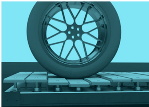
Fig. 2. Prototype of a speed bump design for energy recovery [7].
