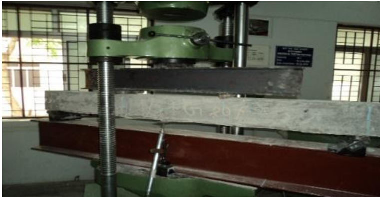
Fig. 4. Two-point loading setup
