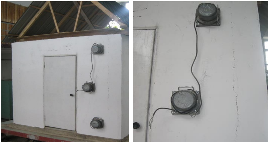
Fig 6. A general view of the "reinforced concrete frame" model of the house, after the experiment.
