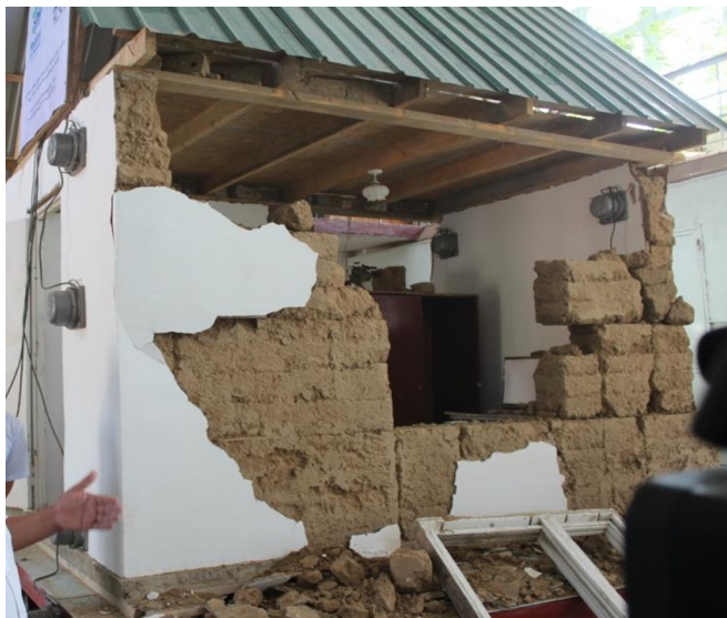
Fig. 1. General view of the model of the house «sokmo» after the experiment
