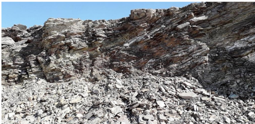
Fig. 3. A sequence of shale beds within the eastern dip, inclined at angles ranging from 20 to 25° degrees, at the face of the southern working slope in the Central quarry.
