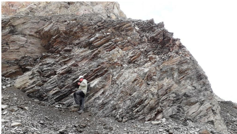
Fig. 2. Thickness clayey shale Eastern fall at an angle of 40° northern entry in career 1A on Central plot.
