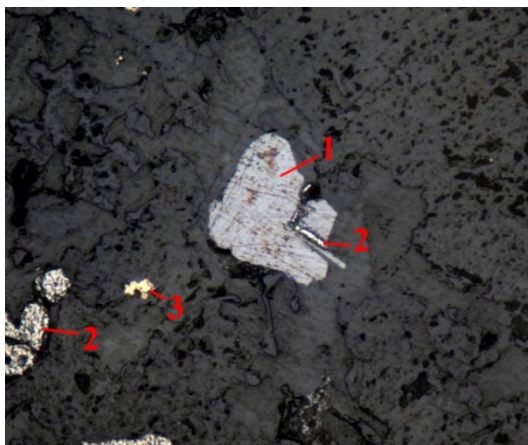
Fig.5. Intergrowth of molybdenite with pyrite. Polished section Yozb-12. Increased 200x. 1-molybdenite, 2-pyrite, 3-chalcopyrite.
