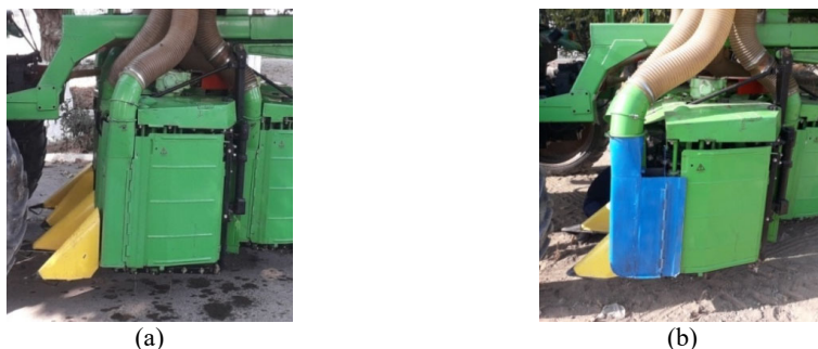
Fig. 2. Vertical spindle machines with serial (a) and new (b) receiving chambers.
