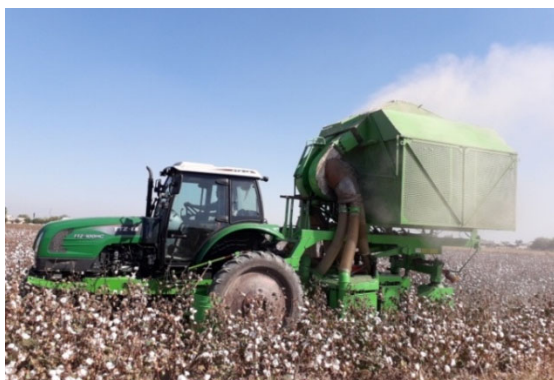
Fig. 3. Separation of dust particles in the hopper of a cotton harvester.
