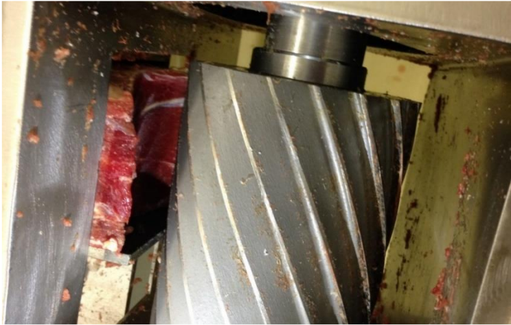
Fig. 14. The contact area between the raw material to be processed and the shredder's working tool (the meat block is moved away from the cutter for clarity).
