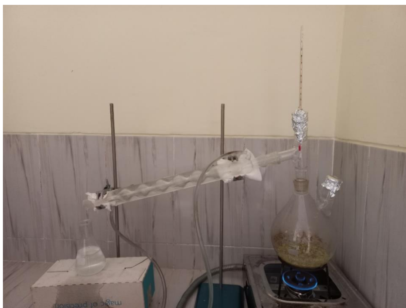
Fig.1 Essential oil distillation process
