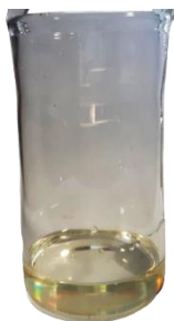
Fig. 3. The clove oil obtained from hydrodistillation of clove leaves.
