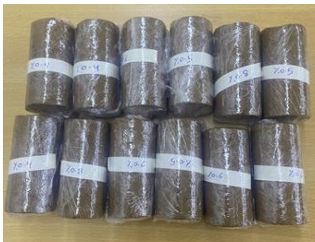
Figure 3: Soil samples prepared with various percentages of nano-MgO.
