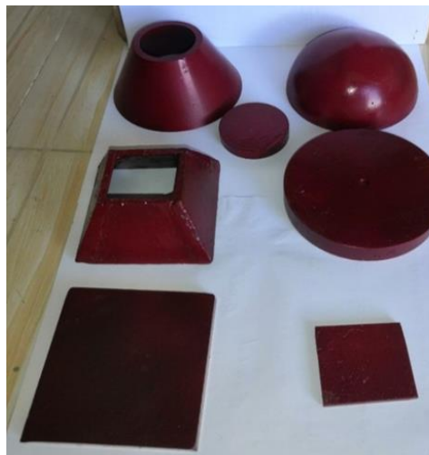
Figure 4: Overall view of shell footing model tested footing models made of steel
