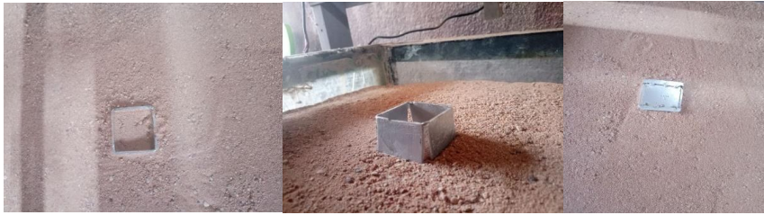
Figure(8): Preparation of the test box for a skirted foundation.
