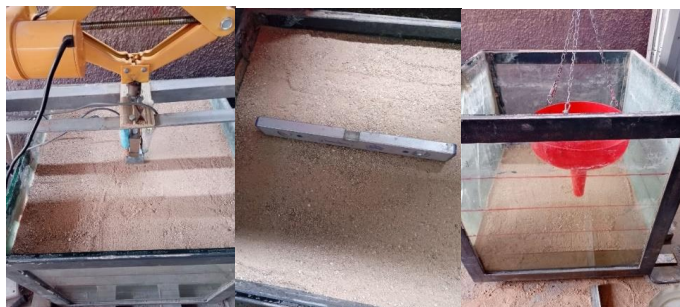
Figure(7): Preparation of the test box for surface footing.
