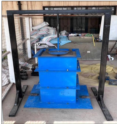
Figure 1: Steel box and loading frame.
