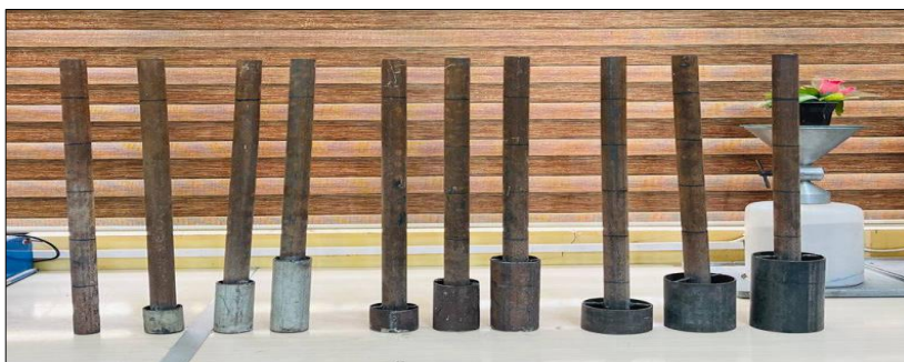
Figure 4: Details of the pile and collar used.
