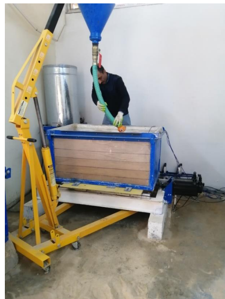
Figure 4: Sand box preparation by raining from the elevated hopper funnel through the diffuser screen.
