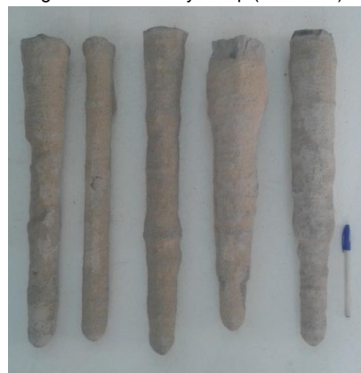
Figure 9: Extracted grouted columns.
