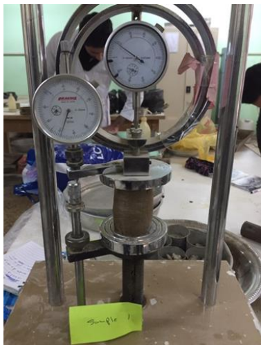
Figure 2: Specimen under unconfined test.
