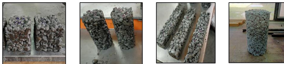
Figure 4: No-fine concrete samples.
