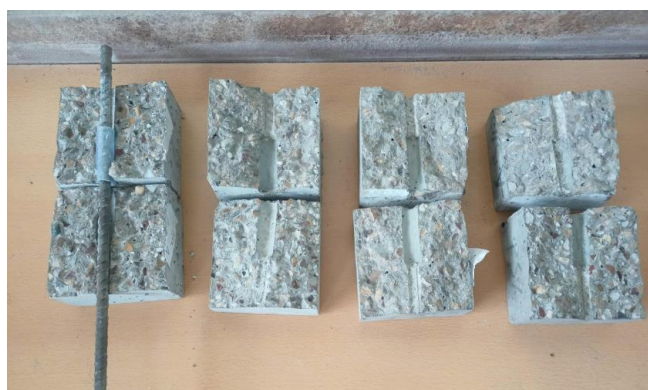
Figure 9: Specimens after failure in bond test.
