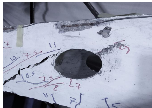
Figure 6: Dapped beam with unstrengthened opening at Failure stage.
