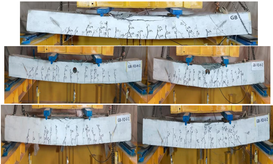
Figure 4: Mode of failure for the tested beams.
