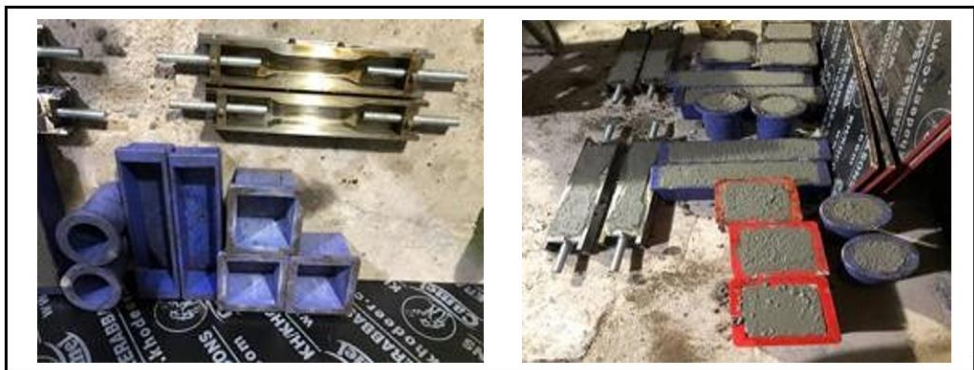
Figure 4: Sample molding for each examination model.
