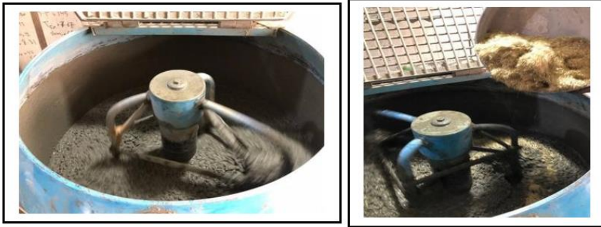
Figure 2: The process of mixing ingredients with a rotary mixer.
