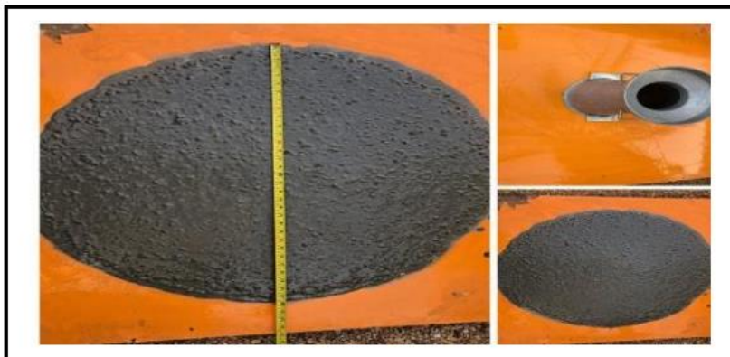
Figure 6: The slump flow test.
