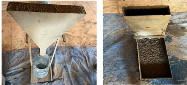
Figure 2: V-funnel and L-box experiments of study mixtures.
