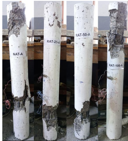
Figure 3: Failure patterns of columns with tied reinforcement.
