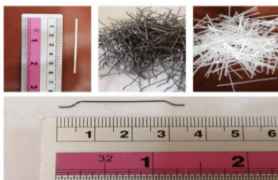
Figure 1: Hooked end steel fiber and polypropylene.
