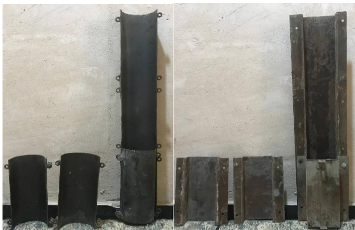
Figure 4: Square and circular iron molds.
