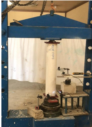
Figure 5: Electro hydraulic testing device of columns.
