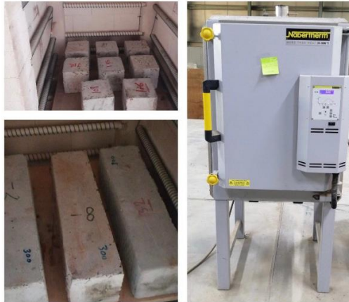
Figure 1: The furnace and Concrete specimens' arrangement.
