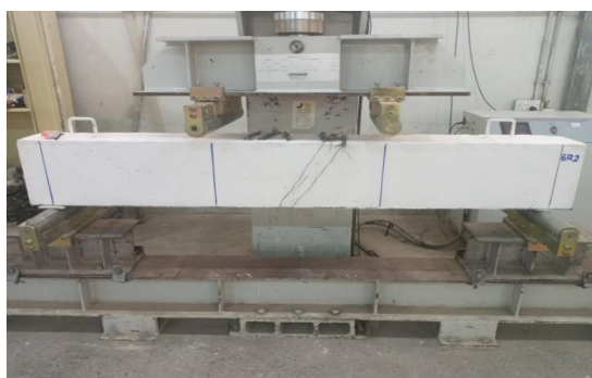
Figure 5: Flexural testing machine.
