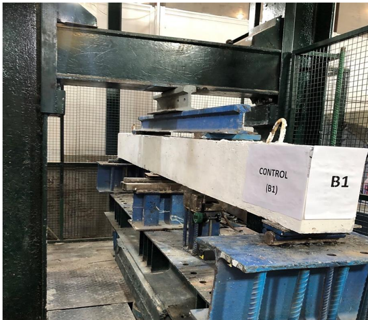
Figure 4: Control under the compression hydraulic machine.
