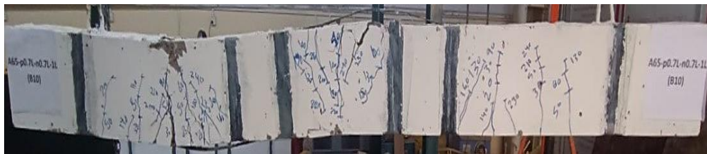
Figure 10: Map of cracks for A65-p0.7L-n0.7L-1L.
